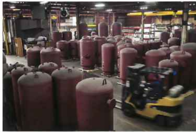
Hot Water Storage Tanks & Buffer Tanks
