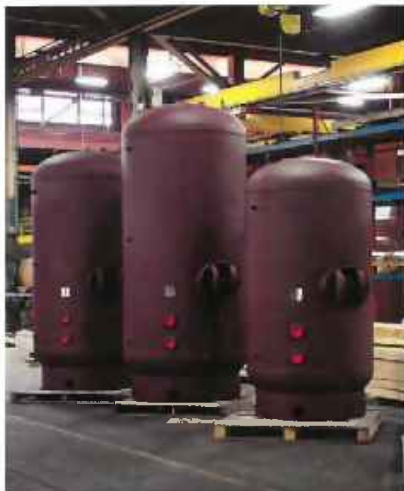
Hot Water Storage Tanks
